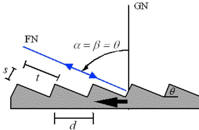
In the Littrow configuration  $\beta = -\alpha$ , and the diffraction condition
