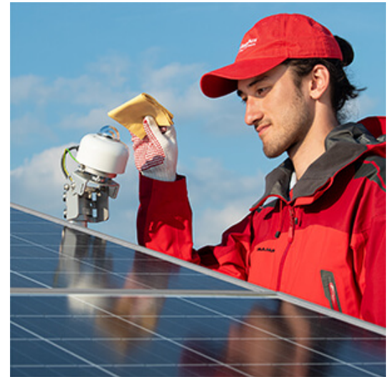
Figure 3 Hukseflux's SR300-D1 pyranometer containing a thermopile sensor to measure the solar irradiance.
