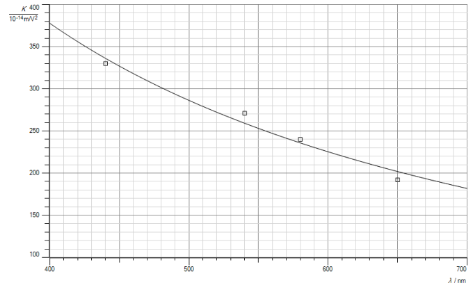
Figure 2: Kerr constant as a function of the wavelength with nitrobenzene
