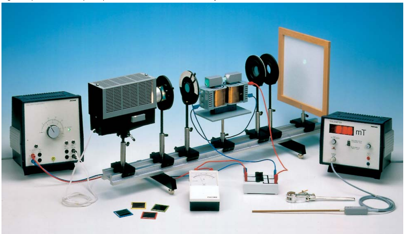
Fig. 1: Experimental set-up for quantitative treatment of the Faraday effect.
