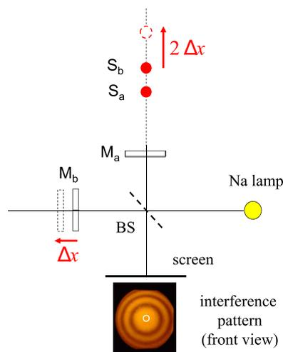
**Figure 2.** Schematic representation of the light paths: a displacement  $\Delta x$  of the mirror  $M_b$  induces an increment  $2\Delta x$  of the optical path. The diameter of the image on the screen is about 3.0 cm; the white circle marks the region seen by the light sensor (provided with a pinhole of 1.5 mm of diameter) during the measurements.
