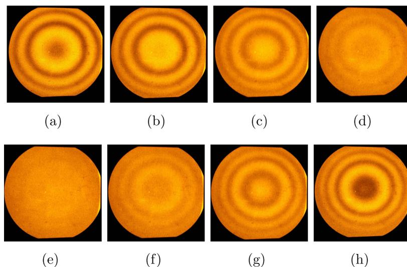
**Figure 3.** Typical sequence of circular fringes observed on the screen: the displacement of the mirror  $M_b$  between (a) and (h) is about 0.3 mm, i.e. 300 turns of the RMS. The diameter of each pattern is about 3.0 cm.
