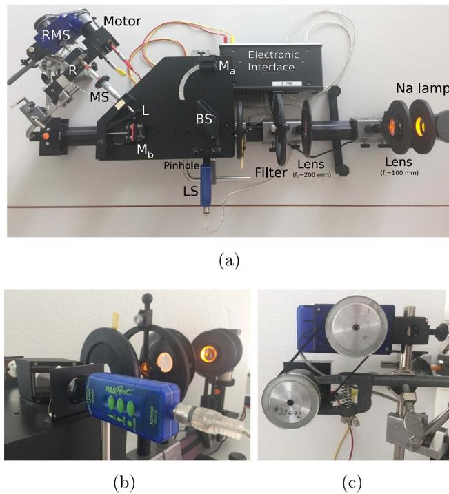
**Figure 1.** (a) Top view of the experimental setup, (b) the light sensor and the optics and (c) the mechanical coupling between the motor and the RMS.
