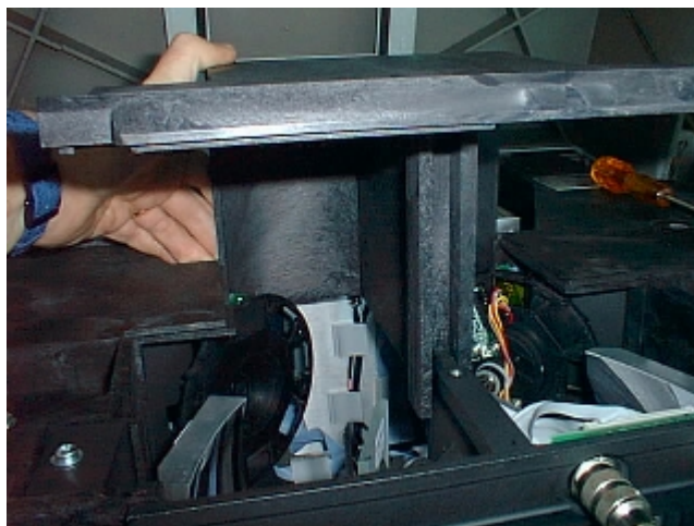
Figure 120 Lifting the cover
