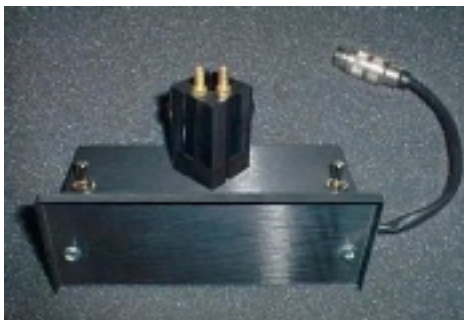
Figure 18 Stirred single position cellholder
