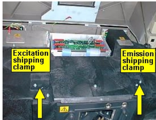
Figure 143 Removing the shipping clamp plates
