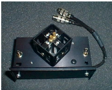
Figure 19 Stirred four-position cellchanger
