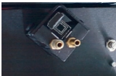
Figure 33 Inserting the semi-micro cuvette
