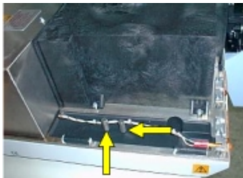
Figure 144 Shipping clamp screws storage positions
