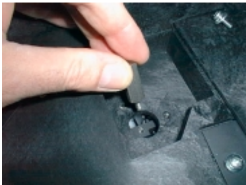
Figure 145 Inserting the shipping clamp screws
