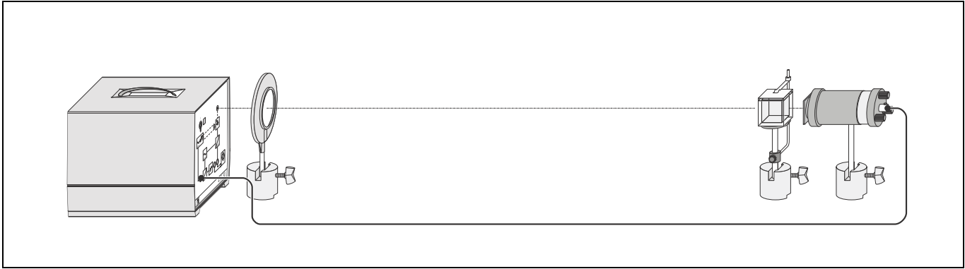
Fig. 5 Determining the velocity of light in organic liquids.
