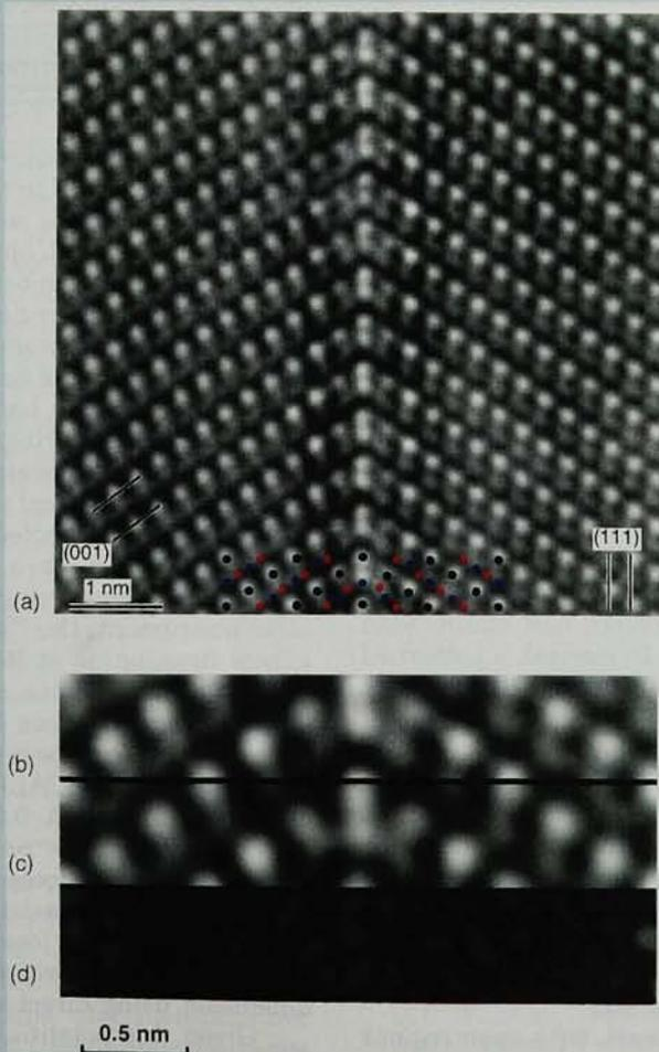
data (b), together with the atomic structure assumed in the simulation (the colored dots), which can be compared with the calculated image (c). The simulation was based on quantitative refinement, and the small residual differences—of order the experimental errors—are displayed in the bottom part of the figure (d).
